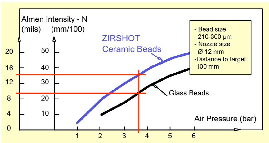
Fig. 1: Due to its higher density, when used in a wet process, Zirshot provides higher mass flow and Almen intensity for the same air pressure (Saint-Gobain ZirPro, ICSP'4, 1990).
