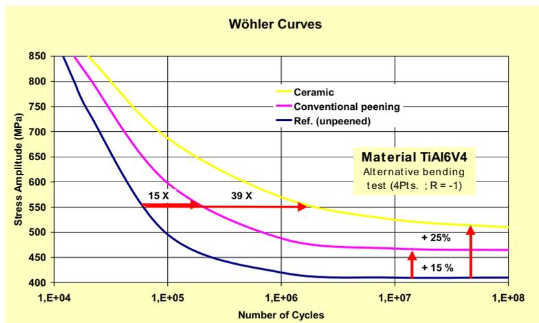
**Fig 4: H.E. Franz, A. Olbricht, ICSP'3, 1987: significant improvement of both life time (40 x) and fatigue strength (+25%).**
