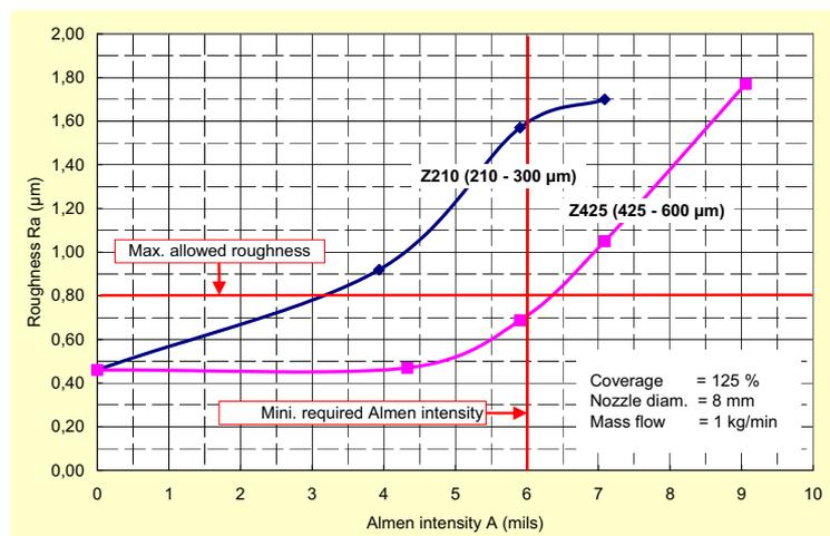
**Fig. 5: Optimisation of Zirshot size according to minimum required Almen intensity and maximum acceptable roughness. Zirshot Z425 is appropriated (Saint-Gobain ZirPro 2001).**
