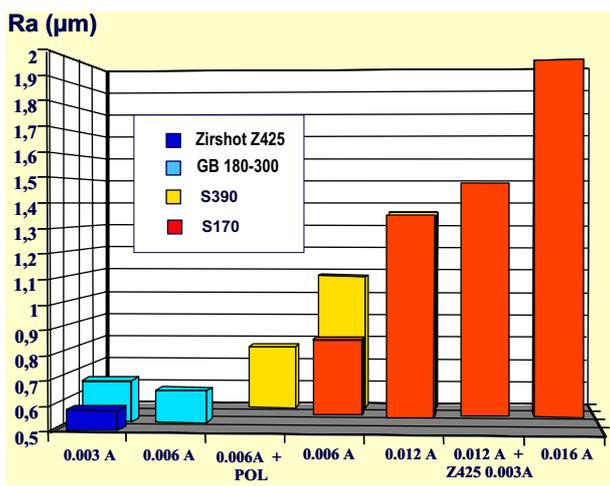
Fig 2: H.E. Franz, A. Olbricht, ICSP'3, 1987: Roughness of titanium after dry peening with several shot types.
