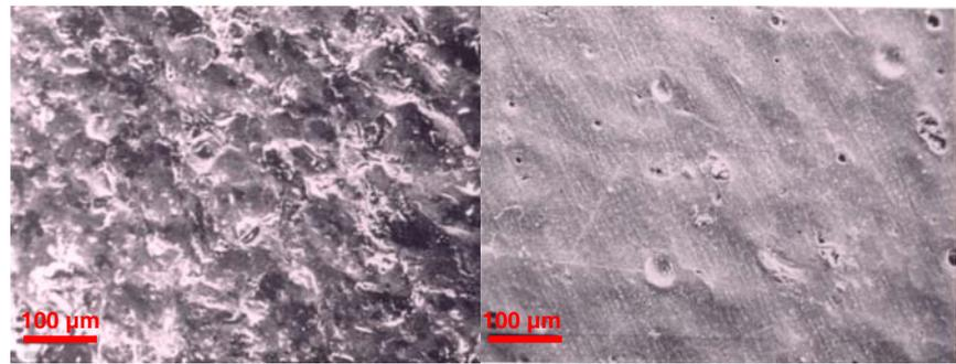
**Pict. 1: SEM pictures of Titanium sample surface after peening with glass beads (left) and Zirshot (right). Magnif. 150 x**
