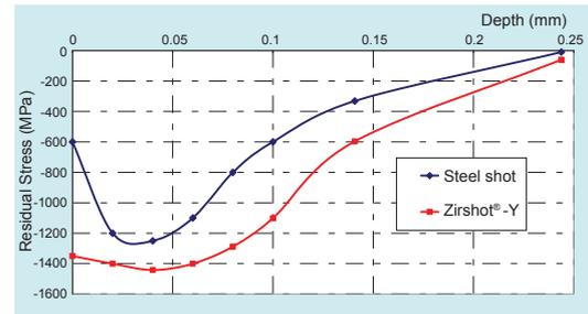
**Chart 3: With comparable depth of compressive layer, residual stress profiles show much higher compressive stress at the surface after peening with Zirshot®-Y ceramic shot vs. Steel shot**
