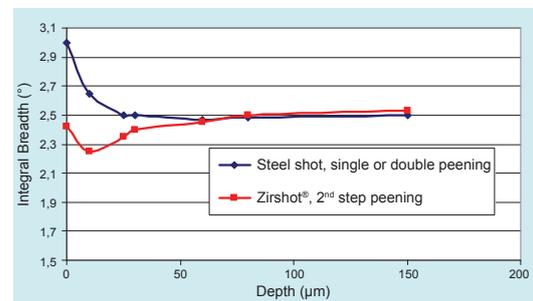
**Chart 5: Dislocation density (integral breadth of diffraction pick) is much lower after peening with Zirshot® vs. steel shot**
