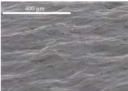
**Picture 2: SEM picture of the surface condition after 2<sup>nd</sup> step peening with Zirshot®. The surface has been smoothed; no more visible surface defect**
