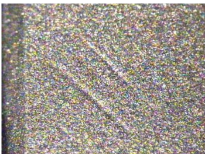
Picture 6: Microscope pictures of a gear tooth surface showing groves after machining (top) and the same place after peening with Zirshot®-Y where groves have been "repaired" (bottom)
