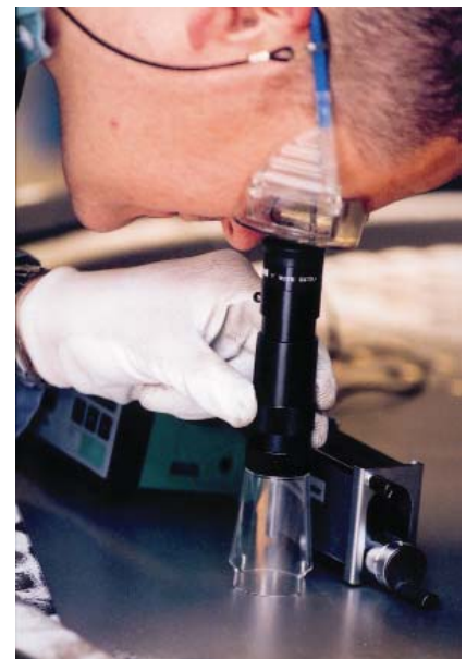
Surface inspection after shot blasting
