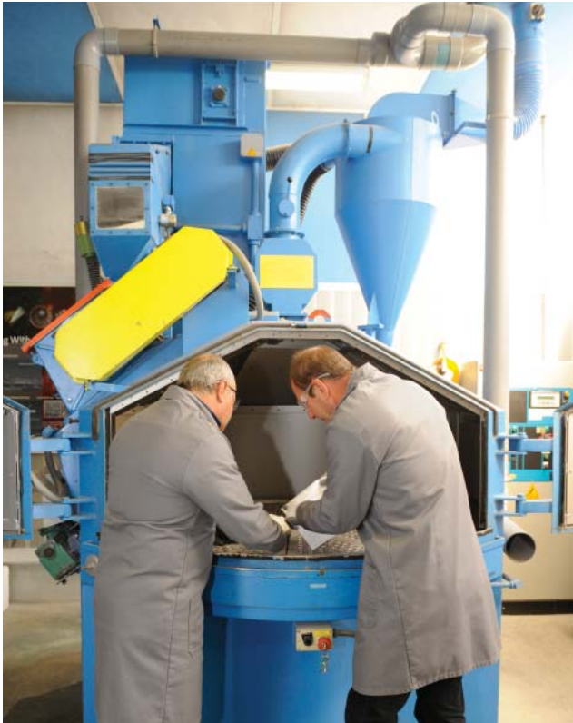
Turbine blasting tests at ZirPro's application shop
